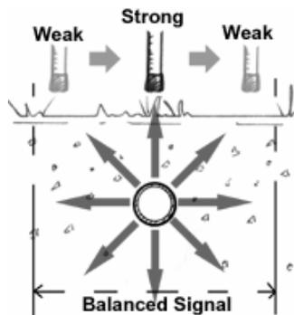
While locating always hold the Receiver vertically, and in the direction of the pipe (in-line with the handle). Swinging the Receiver as you scan may lead you to interpret the signal incorrectly.
