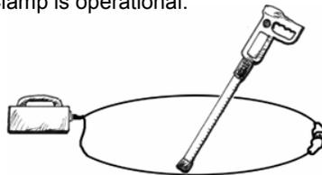
If the locator fails the checks above, or if the Transmitter makes a beeping tone, or if the Receiver's volume is low, replace batteries and repeat checks. If it fails again with good batteries, the locator may need repair.
