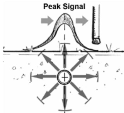
Be careful when on a hill or steep bank. Try to keep the Receiver level, not parallel to the hill. The Receiver will go towards the strongest tone, and if it is kept parallel to the hill side that tone will **NOT** be directly over the conductor as shown below. The deeper the conductor is, the worse this problem becomes.
