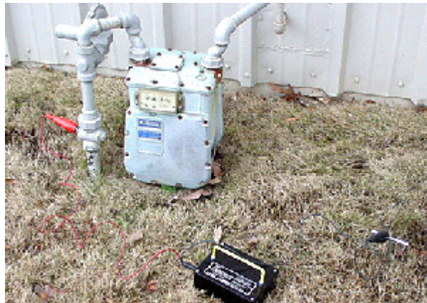
LF Transmitter Conductive Setup
