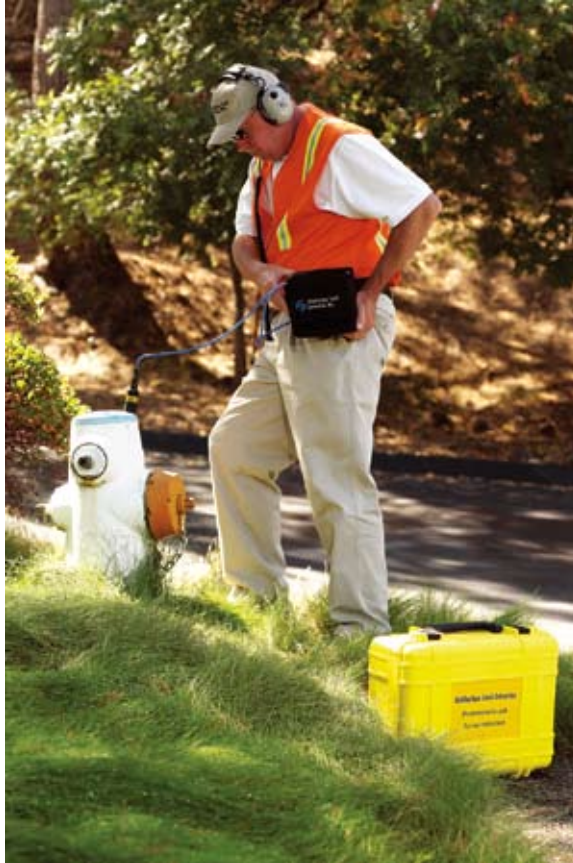
Surveying at a hydrant with the sensor and magnet
