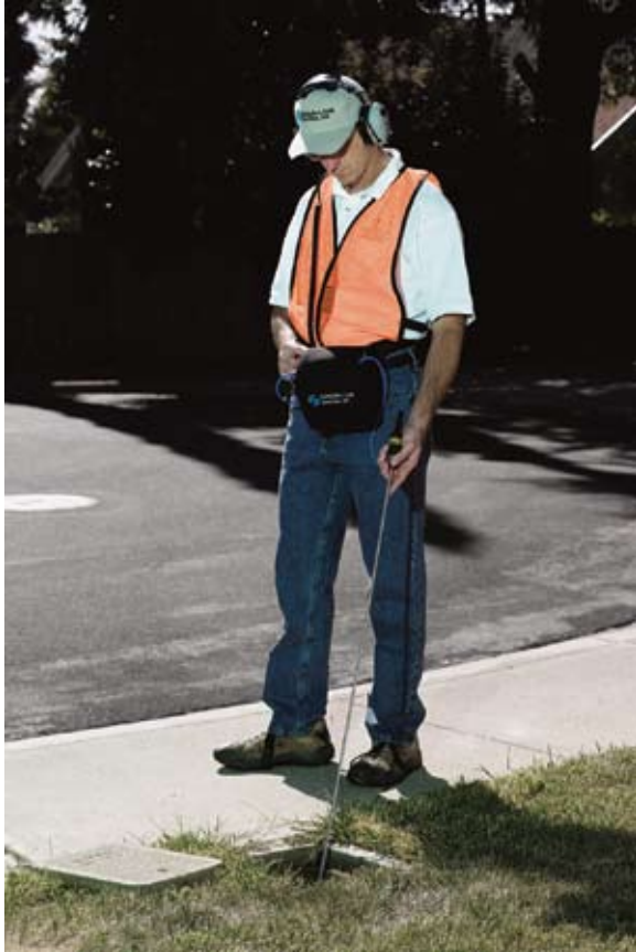
Surveying at a meter with the optional contact rod
